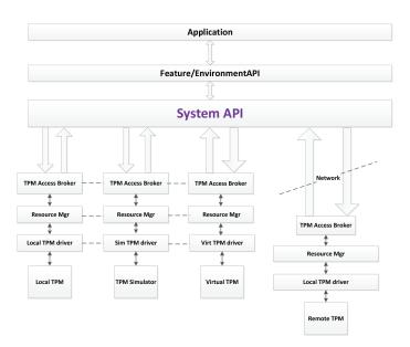
The diagram above shows where the TPM 2.0 device fits in the TSS stack.
