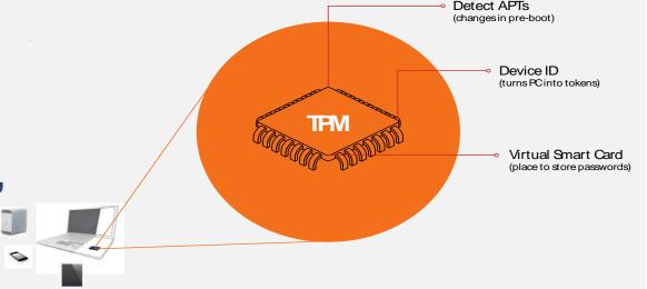
A secure micro-controller with cryptographic features that provides a root of trust enabling the secure generation of keys and the ability to limit their use for encryption/decryption & signatures, and as a secure container for key storage.
