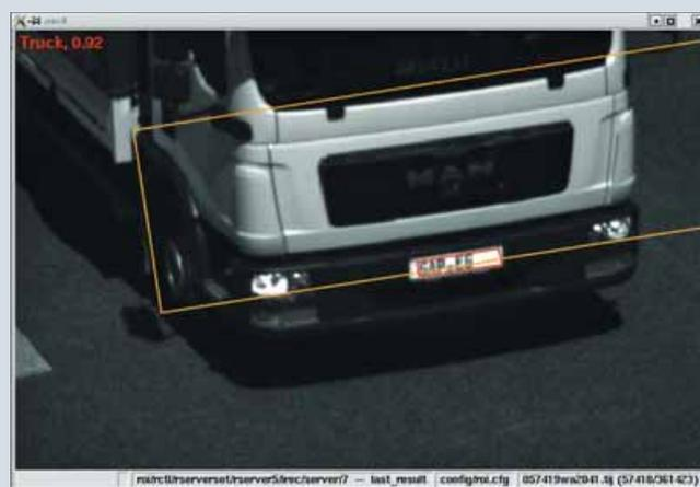
... and selects the picture detail that allows optimum number plate recognition
