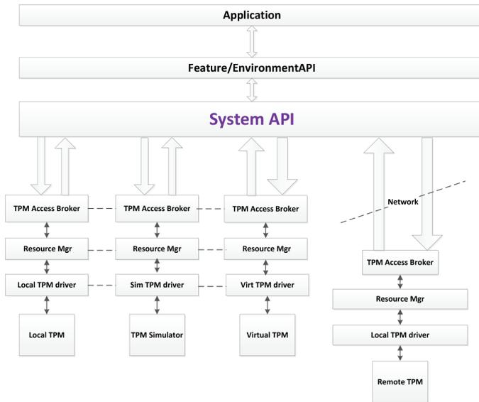
*The diagram above shows where the TPM 2.0 device fits in the TSS stack.*
