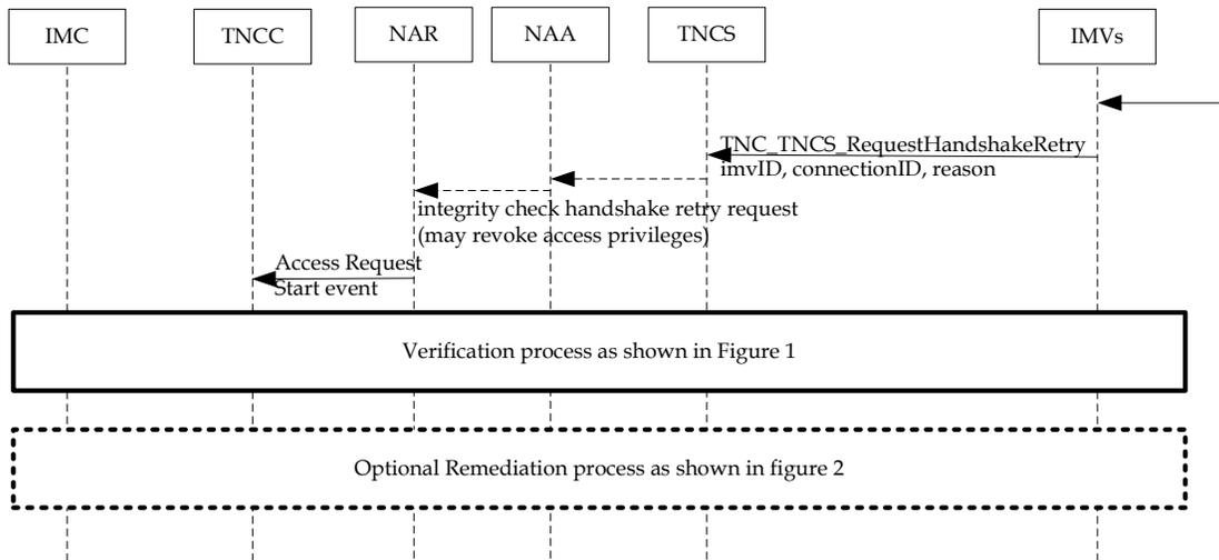
Figure 3 – C Bindng: IF-IMV Handshake Retry Initiated by TNCS
