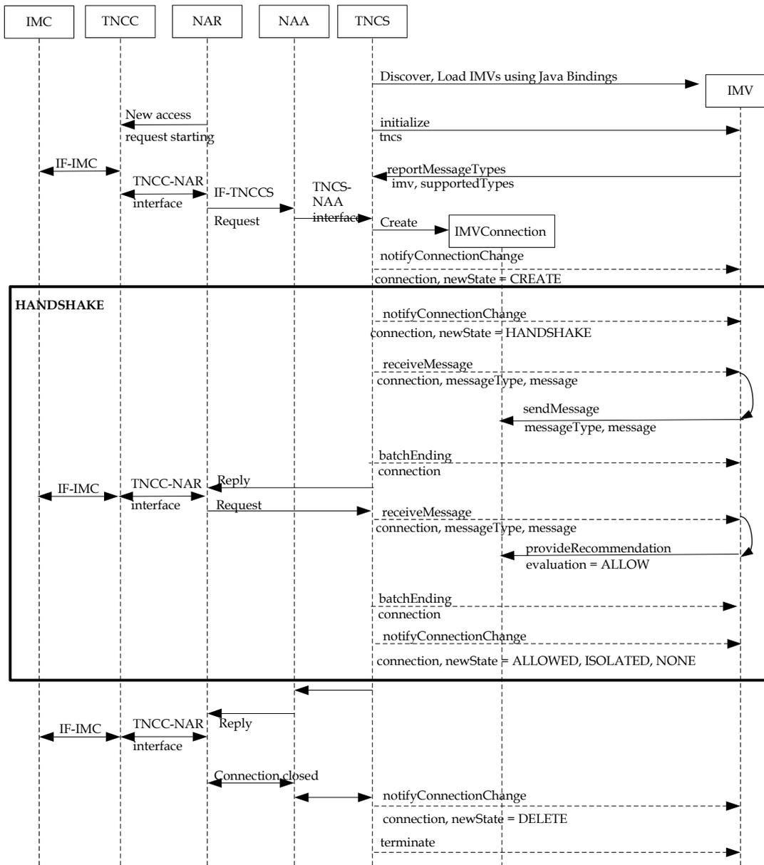
Figure 4 – Java Bindings: IF-IMV Network Connect Sequence Diagram
