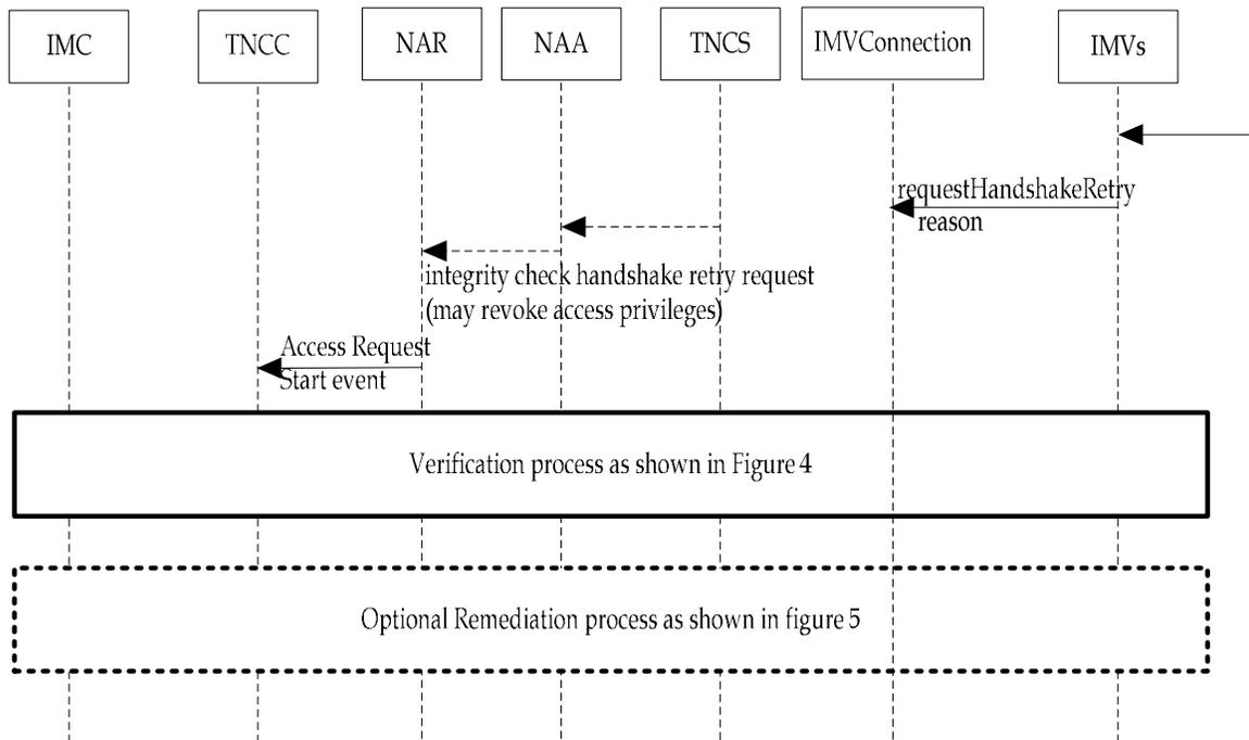
**Figure 6 – Java Bindings: IF-IMV Handshake Retry Initiated by TNCS**
