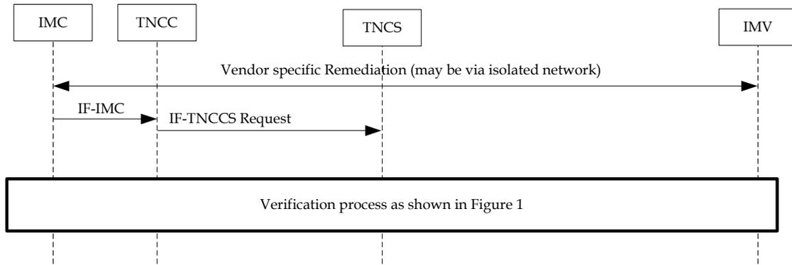
Figure 2 – C Binding: IF-IMV Handshake Retry After Remediation Sequence Diagram
