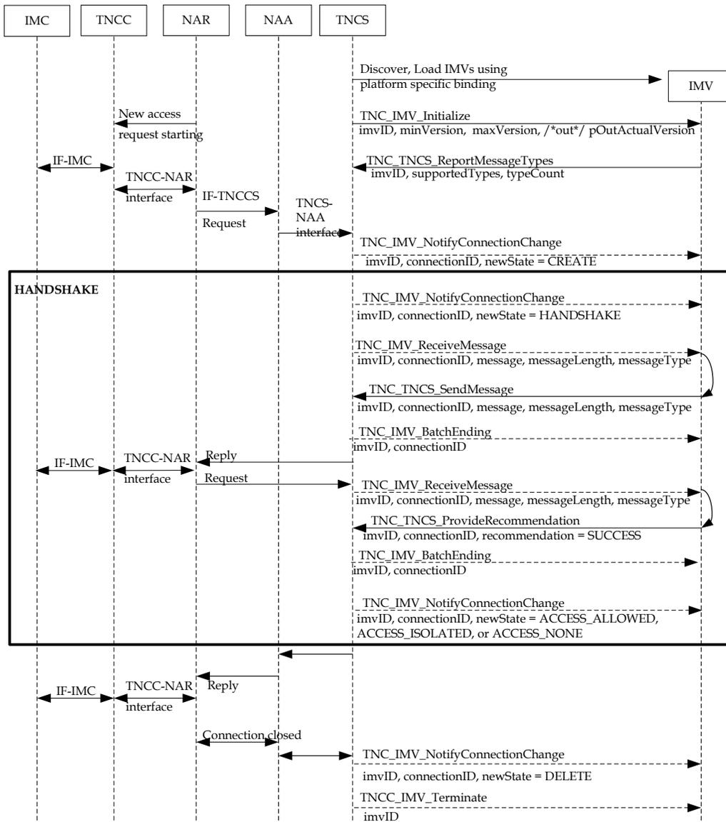
Figure 1 – C Binding: IF-IMV Network Connect Sequence Diagram
