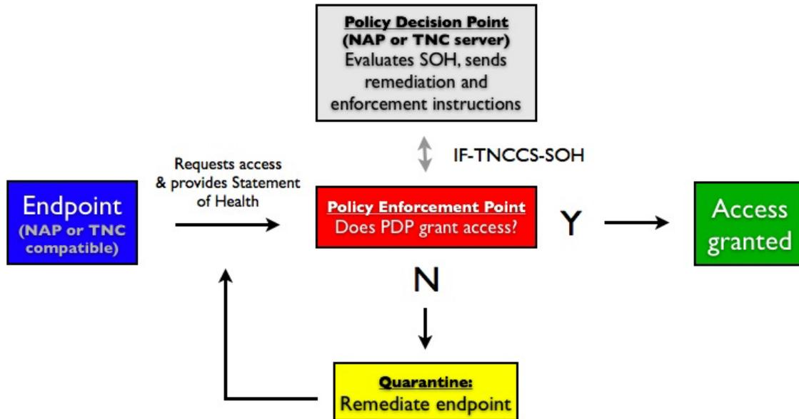
*In either a TNC- or NAP-protected network, endpoints must share their state of health (SOH) information. Endpoints which comply with health policies (specified by the PDP) receive relevant access (via the PEP). Endpoints which fail are shunted into a network quarantine with limited access, until remediated and reassessed.*
